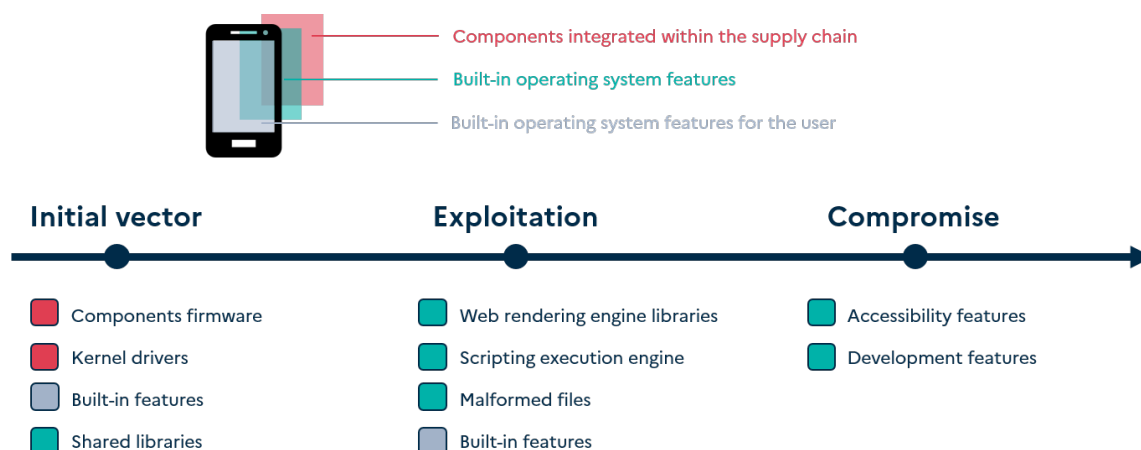
Figure 3: Examples of exploitation of OS built-in components in an exploit chain
